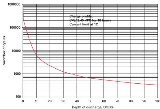
The true dual purpose design of ODYSSEY batteries is reflected in the cycle life results shown in the graph below. This graph is from an 80% DOD cycle test completed on two ODYSSEY 65-PC1750 battery samples. Both samples gave over 500 cycles before failing to give 80% capacity (this is classified as end of life.)
